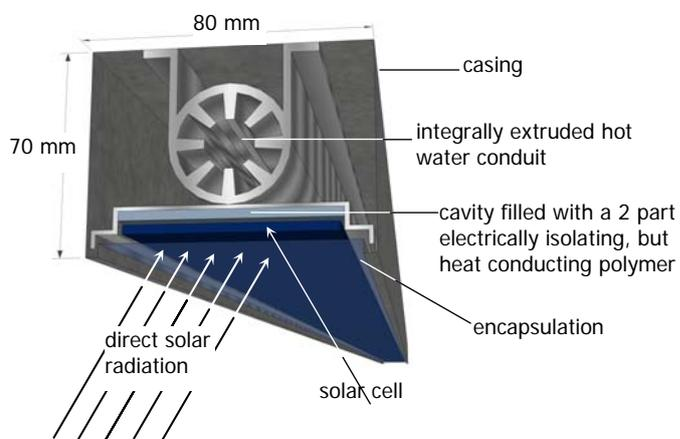
**CHAPS receiver incorporating high efficiency concentrator cells**
