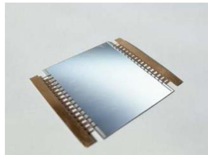
**High efficiency concentrator cell with tabbed bus bars**
